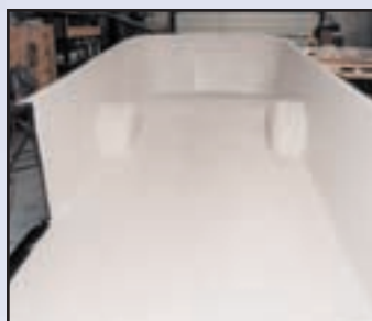
Finished molded lower body/floor pan ready for floor installation.
